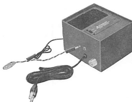
**SR-CMA Mobile master.** This has two functions, combined in the metal case with the magnet mount. The line filter choke is built in the case to avoid the alternator whine trouble, and a UHF female connector on the case to connect the external antenna to the antenna connector on the radio.
