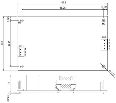
DC Input Connector (CN1): JST B3P-VH-B or equivalent
