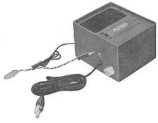
**SR-CMA Mobile master.** This has two functions, combined in the metal case with the magnet mount. The line filter choke is built in the case to avoide the alternator whine trouble, and a UHF female connector on the case to connect the external antenna to the antenna connector on the radio.
